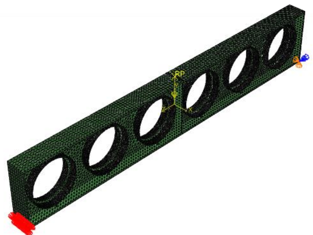
Figure 2: Finite element model with mesh and boundary conditions
