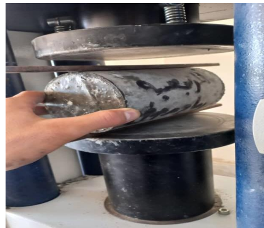
Figure 7: Indirect Tensile Strength Test
