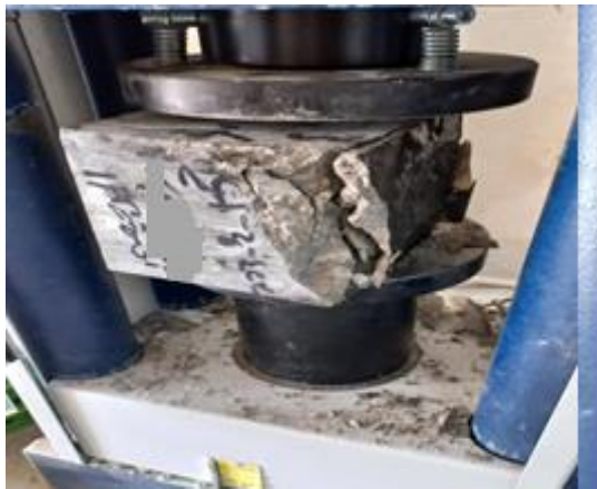
Fig.5: Compressive Strength Test
